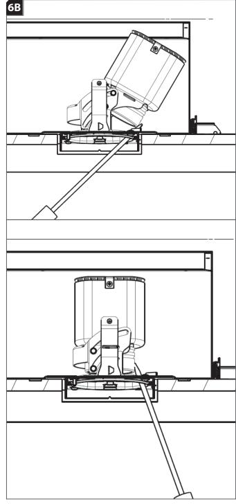
To tilt the module from a tilted position back towards the 0° downlight position, insert a long screwdriver and contact the back of the heat sink. Using a prying motion, tilt the module inward to the desired position.
