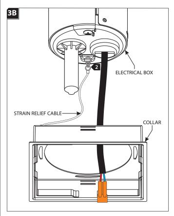
Use the clip to secure the strain relief cable onto the electrical box.
