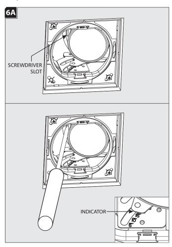
To adjust the module, insert a flat head screw driver into the slot of the module and gently pry the module to the desired angle.
