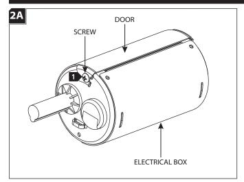
Open the electrical box door by unscrewing and removing the two screws using a screwdriver.
