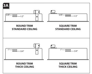
Identify the correct collar for your ceiling thickness. The shorter collar is used for 1/2"- and 5/8"-thick ceilings, and the taller collar is used for 3/4"- and 1"-thick ceilings.
